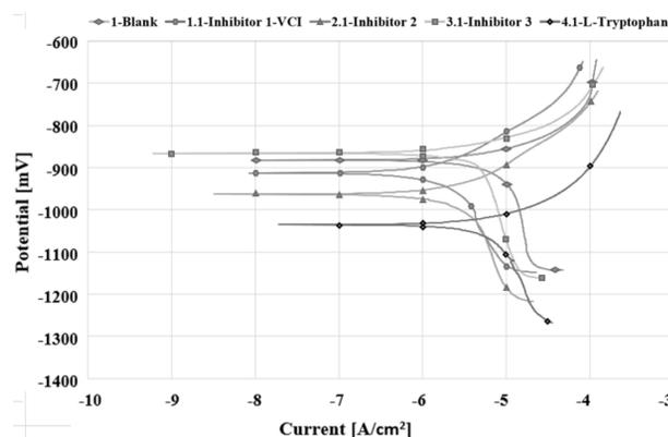
Figure 1. Polarization curves of tested inhibitors, compared to unprotected galvanized steel in fresh water
