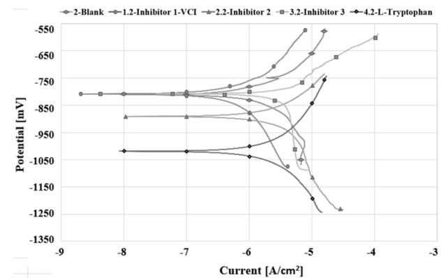
Figure 2. Polarization curves of tested inhibitors, compared to unprotected galvanized steel in distilled water
