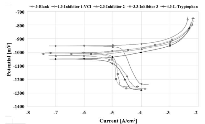
Figure 3. Polarization curves of tested inhibitors, compared to unprotected galvanized steel in 1% NaCl solution
