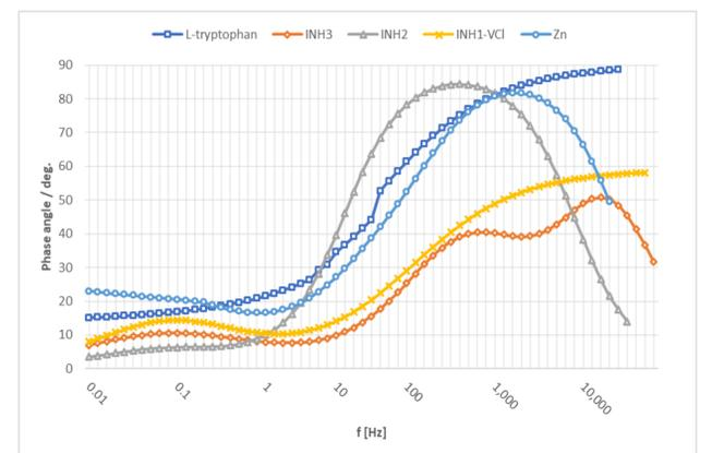
Figure 4. The Phase angle diagram of all tested samples 24 h immersion in 1% NaCl solution
