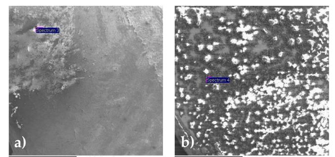
Figure 5. SEM view of inhibitor layer after 24 hours in distilled water; a) Inhibitor 1-VCI and b) L-Tryptophan
